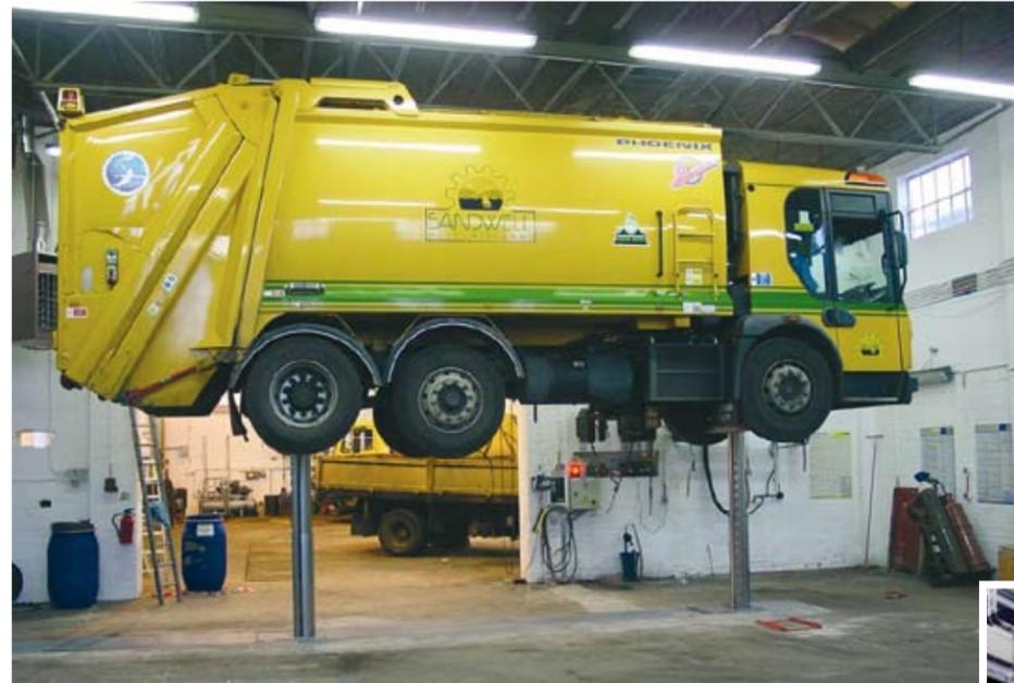
Exchangeable sliding supports allow to lift all types of vehicle of the appropriate weight category with a maximum of safety.
