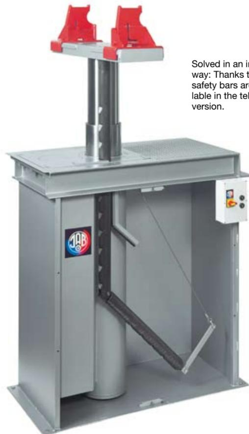
Solved in an intelligent way: Thanks to the joint, safety bars are also available in the telescopic version.
