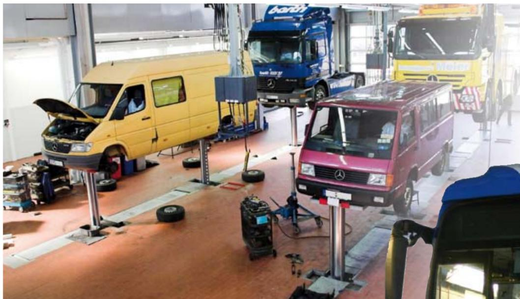
2 HVV four-ram-lifts, which are used as 2 two-ram-lifts.
